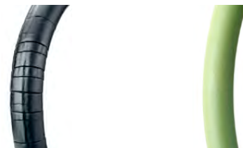
O-rings in nitrile (left) and viton after test at 200° C.
